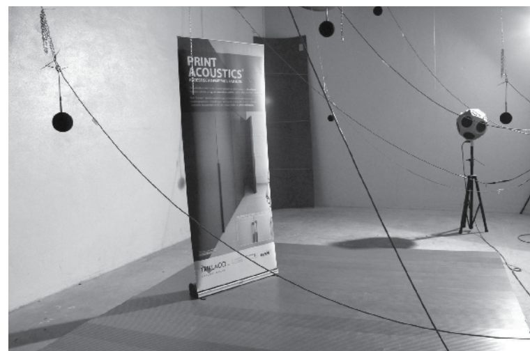
Test set-up in lab - EN ISO 354:2003
